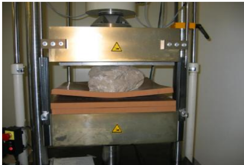
Figure 2: Setup of the experiment, showing the Hydropuls testing device, the stone representing the head of the statue and the elastic bedding with Sylomer M75
