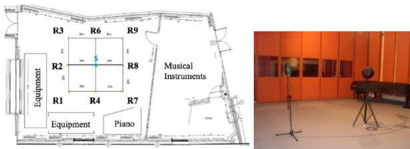
Figure 2 a) Floor plan of the live room. The receivers and source positions for this study are marked at the front (largest) part of the divided space by the sliding rail, b) The dummy head and the omnidirectional source during the measurements at position R6.
