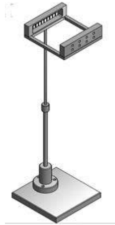
Fig. 1. A two-dimensional optoelectronic sensor for recording flying insects' wingbeat inside insectary cages. The receiving surface houses 20 photodiodes aligned as two linear layers of 10 diodes each. The emitter consists of 8 infrared LEDs. Dimensions of the rectangular passing through window, is 9 cm.
