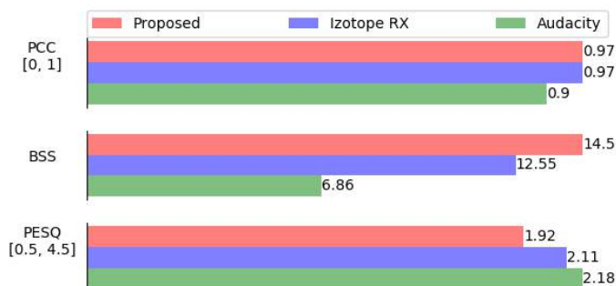
Figure 0.4 Evaluation metrics comparison between proposed framework and third-party tools. (file used: sp01_car_sn10.wav). Highest score is better.
