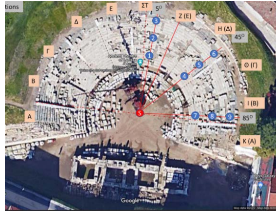
Figure 1.1 Top view of the theatre showing the measurement positions (blue dots) and the sound source position as the red dot [6]
