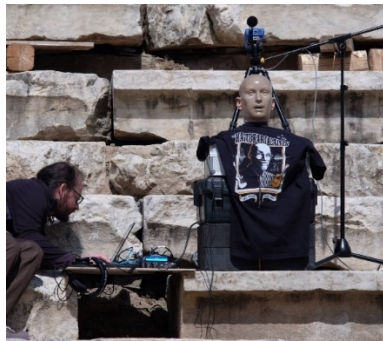
Figure 1.2 Preparation of the measurement setup. It consists of the KEMAR binaural dummy head, the omnidirectional microphone and the SPL meter.
