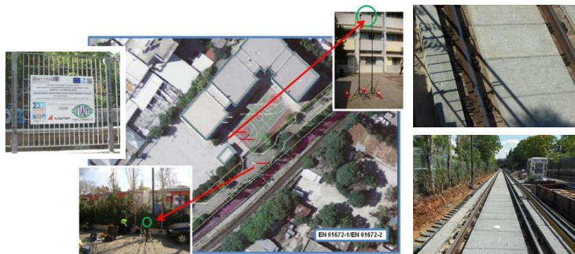
Figure 2.2 Implementation of "SoundSorb" in the Test area & Measurements location according to EN ISO 3095:2005(E) with monitoring equipment according to EN 61672-1/EN 61672-2
